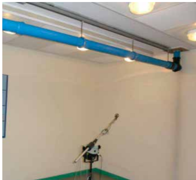
Photo 6 Measurement of the air-borne noise
