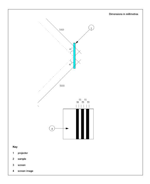
A grid pattern slide, when projected onto the screen must give dark and clear stripes measuring 55 mm wide. Stripe width is calibrated using a non-distorted front surfaced mirror in place of the specimen.
