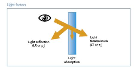
Mirox 4Green is opaque thanks to its paint. Its opacity is measured with a lux meter (HD 2102-2-Probe 471) and a spotlight. Only 0.0002% of light (lux) passes through Mirox 4Green. In a standard mirror, 0.1% of light passes through.
